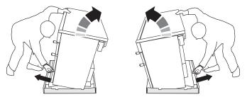
Repeat from the back and remove the rear half of the poly base.
